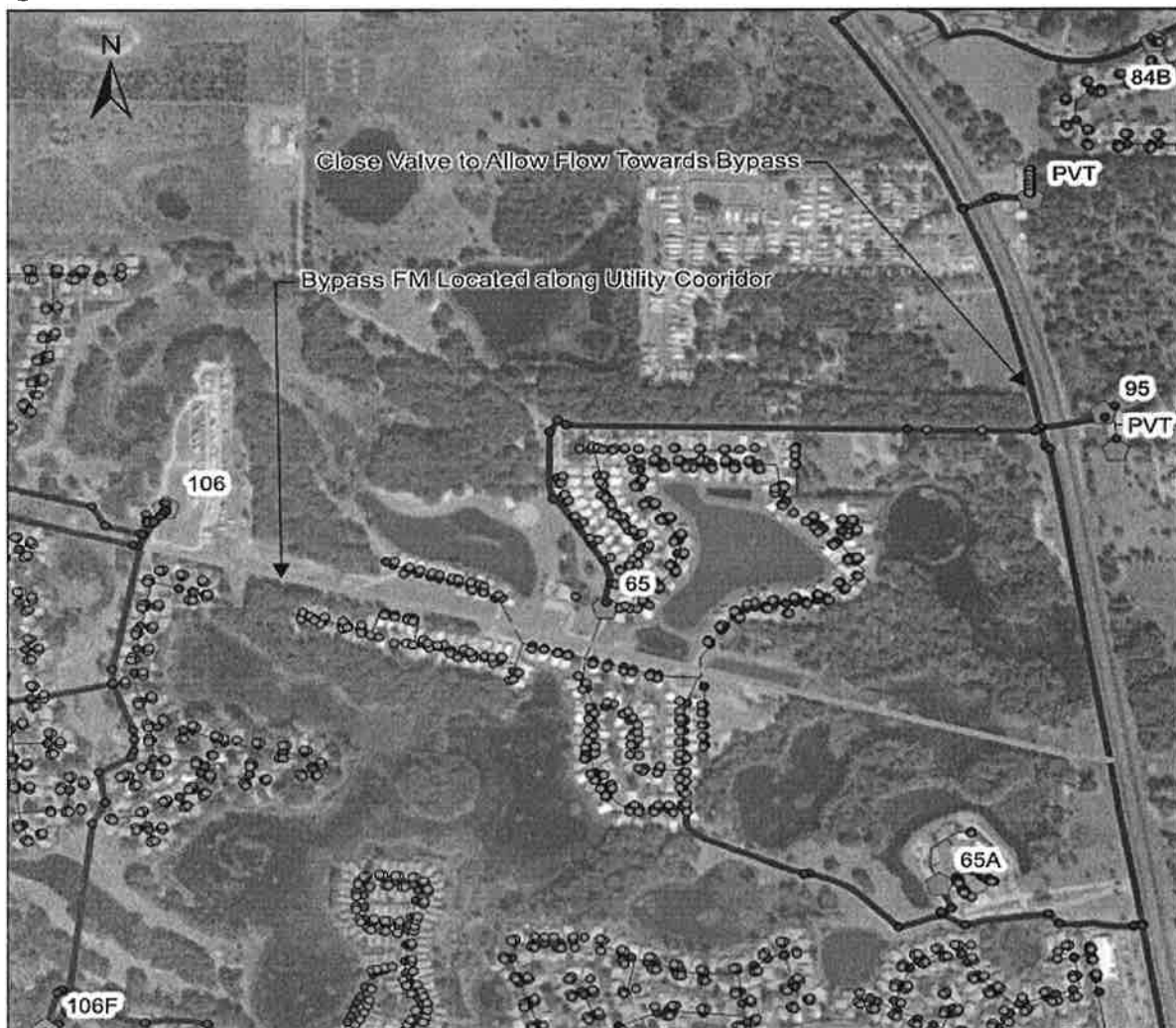
Figure 1 Fall 2020 Lift Station 72 By-pass Force Main Layout
